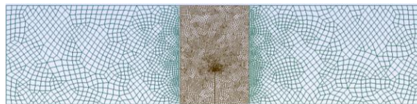
Figure 2. Discretized geometry of the notched concrete beam
